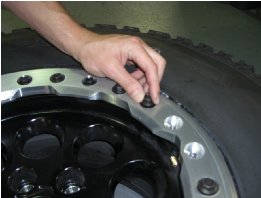
Pic 6.1 – Hand thread in all remaining bolts.
