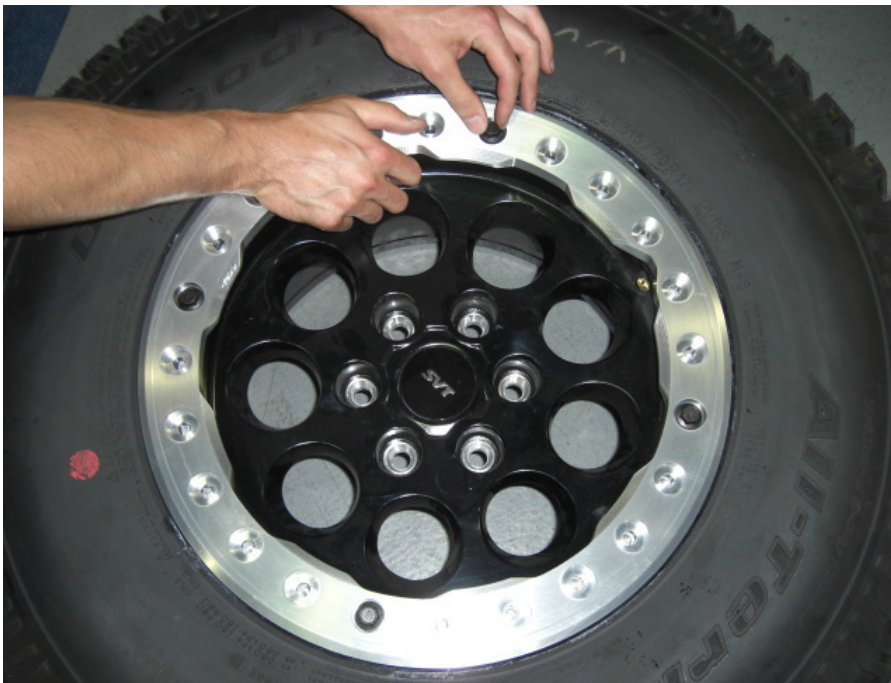
Pic 5.1 – Hand thread 4 bolts at the corners.
