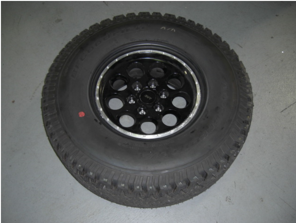
Pic 3.1 – Outer tire bead fits on wheel flange.
