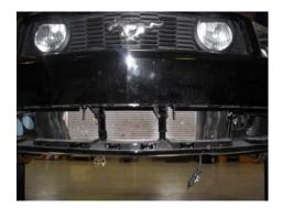
**STEP 9:** Gently unclip both foglight delete bezels from outboard sides of lower grille insert and remove.
