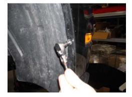
STEP 6: Remove (4) inner fender liner push retaining clips and remove front half of inner fender liner on each side.
