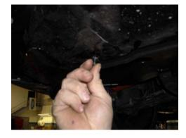
**STEP 5:** Remove (2) front side inner fender liner bolts per side.
