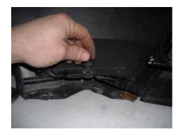
**STEP 8:** Gently unclip lower grille insert from fascia and remove by sliding forward.
