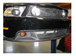
STEP 24: Prior to lowering vehicle, inspect clearance to brake cooling ducts by turning steering wheel lock to lock in both directions. Check for interference to moving parts and ensure duct free-play is correct each side.
