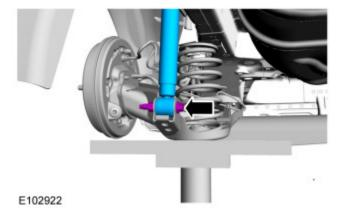
STEP 4: IMPORTANT NOTE: Tighten the shock absorber lower bolt while the suspension is at curb height or bushing damage and incorrect clamp load may occur.
