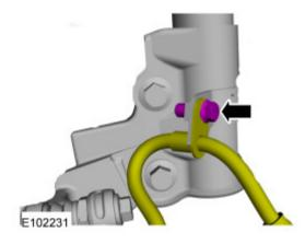
STEP 8: Remove the wheel knuckle-to-strut nuts, bolts and the strut and spring assembly.
