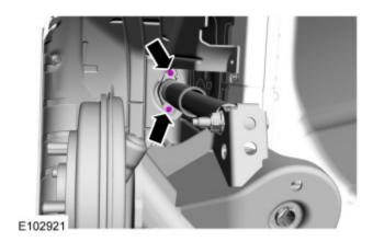
**STEP 3:** Remove and discard the shock absorber lower bolt and remove the shock absorber.
