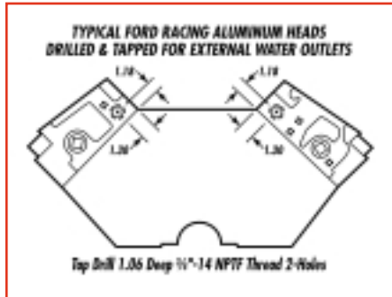
TYPICAL FORD RACING ALUMINUM HEADS DRILLED & TAPPED FOR EXTERNAL WATER OUTLETS Top Drill 1.06 Deep 1/4"-14 NPTF Thread 2-Holes
