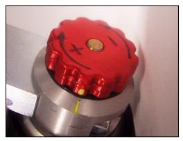
The **compression adjustment** on the **front strut** is a knob on top of the remote reservoir, which is piggybacked to the strut body. It is accessible through the front wheelwell.
