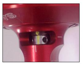
The **rebound adjustment** on the **rear shock** is located in the lower shock eye. It is accessible from under the vehicle, and can be adjusted using a small pin to rotate the adjuster; each hole is 1/4 turn, and the sweep of the eye (the maximum amount that can be adjusted without repositioning the tool) is also 1/4 turn.
