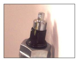
The **rebound adjustment** on the **front strut** is on the top of the piston rod and has a <u>**4mm**</u> hex head. It is accessible from under the hood, and marked in 1/4 turn increments
