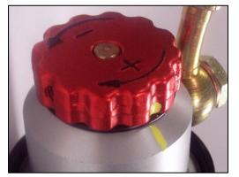
The **compression adjustment** on the **rear shock** is a knob on the remote reservoir. It is accessible through the trunk.
