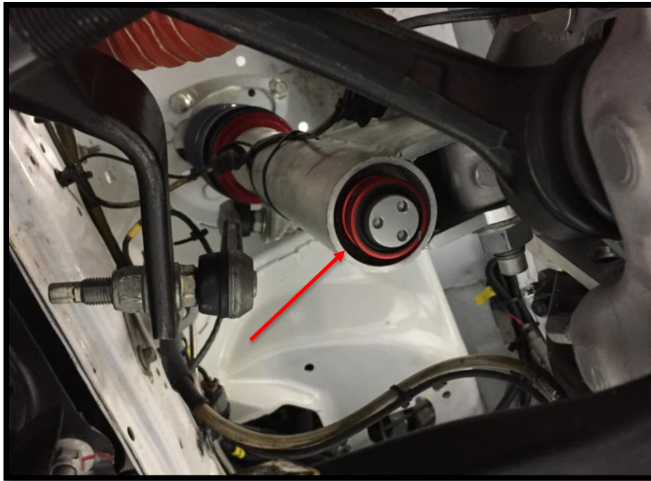
Figure 18: Front rebound adjustment. Clockwise = more damping
