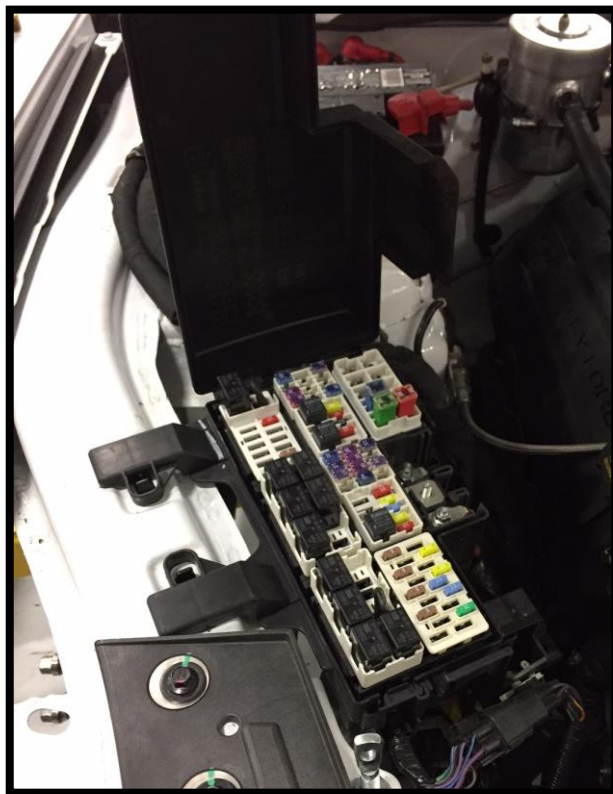
Figure 14: Vehicle Power Distribution Block (PDB)
