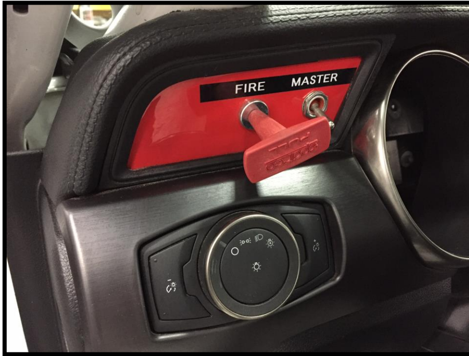
Figure 1: Master Power Switch and fire handle
