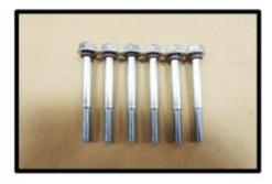
Using 6mm allen socket, secure the (1x) 8mm x 70mm SHCS to pull SC forward to plate. Torque to 22 lbs-ft. NOTE: Failure to do so could cause belt alignment issues.
