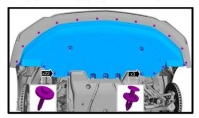
12. (DARK HORSE) Remove the (24x) fasteners and (3x) push pins from underbody shield.
