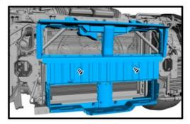
24. (Vehicles equipped with active shutter grilles) Release the tabs and remove upper linkage.
