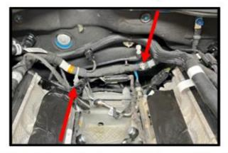
Install supplied TMAP pigtail to stock connector at rear of engine. Route to LH side of vehicle for later installation to supplied 3-Bar TMAP sensor.
