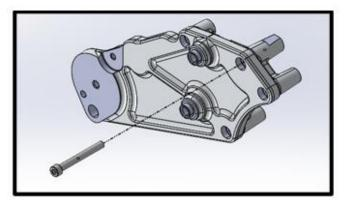
93. Torque (10x) 6mm HHFCS manifold bolts in the following pattern using a 10mm socket. First pass: 88 lbs-in. Second pass: 106 lb-in. **NOTE**: For bolt #10, a 1/4" socket with 4"-6" extension, 10mm wobble is the best possible tool to get into this tight area.
