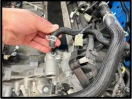
(Auto Transmission) Release the hose clamp from transmission fluid valve and hose facing down from tee. Remove plastic hose retainer from oil cooler solenoid hose.
