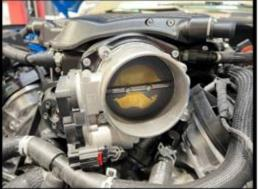
137. Connect previously installed throttle extension pigtail to the throttle body electrical connector. Secure wiring using zip-tie. NOTE: Failure to secure wire may result in the wire catching the belt system!
