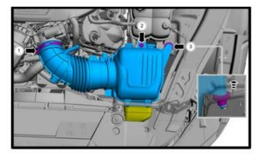
Disconnect the electronic throttle electrical connectors by pushing up on the safety lock and then squeezing the connector and pulling away. Remove the harness retainer from manifold.
