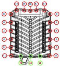
Install (4x) 2-117 IC fitting orings to the (4x) IC fittings. Apply grease to the (4x) 2-117 IC fitting orings. Slide fittings into lid. Secure fittings with supplied fitting retainer bracket and (2x) 6mm x 12mm SHCS bolt. Torque to 80 in-lbs.
