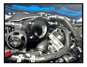
Install supplied (1x) #2-045 V75BR oring to TB adapter. Install the stock throttle body using the (4x) 6mm x 35mm
