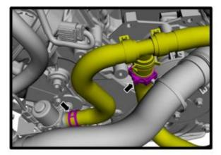
(Auto Transmission) Detach wiring harness retainer from transmission fluid valve bracket. Disconnect valve 2-way connector. Remove the fasteners to remove valve from engine.
