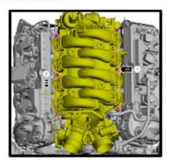
45. Disconnect the engine wiring harness electrical connectors and detach the retainers. Remove intake manifold.
