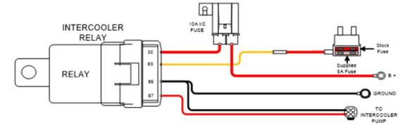
128. Mount relay and fuse holder to the factory airbox stock fastener, secure with zip-tie. Route 2-wire connector down, below radiator, along sway bar to the LH side of the vehicle. Connect to IC pump. Secure harness using zip-ties along bottom of vehicle.
