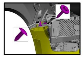
Remove the radiator sight shield by removing the (8x) push pins. Use a flat head screwdriver to pry the center head up. These will all be reused.
