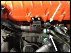
108. Install supplied 3/8" ID x 5 ½" with 55deg quick connect fitting hose (#5000030) to the EECPV barb fitting and **LH** quick connect fitting on SC inlet. Push until it clicks and locks into place.
