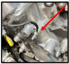
Using 10mm socket, remove the stock fastener (1x) from the top of the RH timing chain cover. Relocate stud with ground wire to the top timing chain cover location. Torque to 22 lbs-ft.
