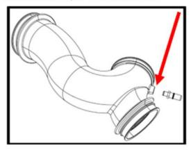
139. Install factory MAF sensors to the new MAF housings using supplied (4x) 4mm x 10mm SHCS. Torque to 17 lbs-in. \*\*DO NOT USE STOCK BOLTS\*\*. \*NOTE: Verify arrow position for airflow direction.
