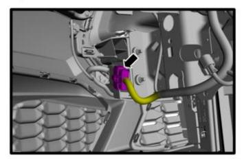
15. On both sides, remove the front bumper cover to fender <u>push-pin</u> and the bolts.
