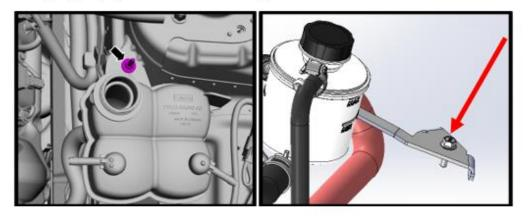
116. Mount IC reservoir to bracket using (2x) 6mm x 12mm HHFCS.
