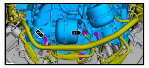
Clean the intake manifold to cylinder head surface using carb cleaner or acetone. Install tape over the exposed ports
