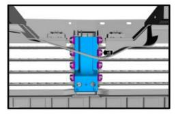
25. Vehicles equipped with active shutter grilles) Release the tab and remove the vane.
