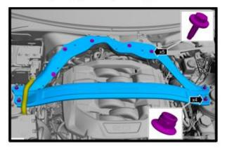
(RHD ONLY) If equipped, remove the strut tower brace by detaching the battery wire retainer. Remove the (4x) nuts and (6x) bolts. Reinstall factory nuts (4) and torque to 41 lbs-ft.
