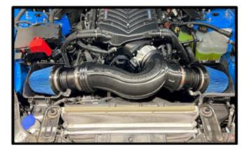
143. Install supplied ½" x 13 ¼" make up air hose to the LH valve cover. Push until it clicks and locks into place. Install other end to air inlet tube fitting previously installed.
