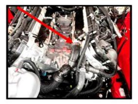
Using 10mm socket, remove the (3x) factory fasteners from the timing chain to head cover and (1x) from water pump (for new idler plate), this includes the factory ground wire/eyelet.
