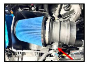
142. Install the inlet tube to the MAFs and throttle body. Secure using the supplied clamps, (2x) #80 on MAF side and (1x) #64 to throttle body. Reconnect MAF connectors to MAF sensors.
