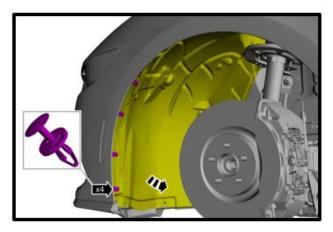
9. (DARK HORSE) On both sides, remove the (4x) fasteners and (6x) push pins from front fender splash shield.
