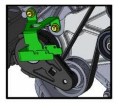
(Auto Transmission) Mount trans cooler solenoid to the supplied bracket using (4x) stock fasteners. Connect extension harness to stock connectors.
