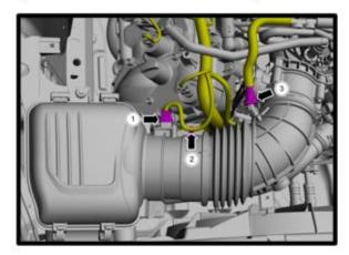
Loosen the hose clamp from throttle body using nut driver. Remove the air cleaner bolt. Detach the air cleaner from grommets and remove the air cleaner.
