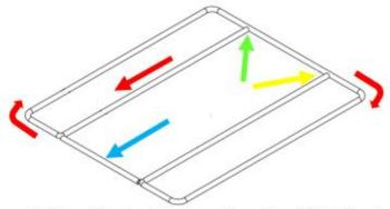
Install supplied pre-formed 65.3" x .103" oring to the top sealing surface of the SC housing. Apply generous amount
