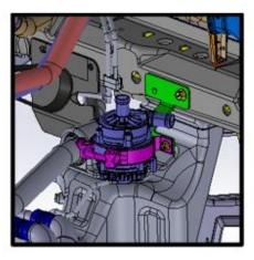
Install hose #3103407 from IC pump to LTR LH low (inlet) fitting. Secure using supplied #16 pinch clamps. Tighten IC pump clamp.
