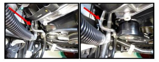
Install the spring-loaded tensioner to idler plate, locating the tang into position. Secure with the supplied (1x) 10mm x 60mm SHCS. Use light amount of anti-seize on threads. Torque to 25 lbs-ft.
