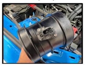
140. Install supplied filters to MAF housing, secure using supplied filter clamp. Install the MAF housings into the Y tube (for ease of installation), pre-install #80 hose clamp to Y tube, leave loose until later.
