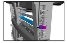
26. Vehicles equipped with active shutter grilles) Remove the bolt and the active grille shutter actuator.
