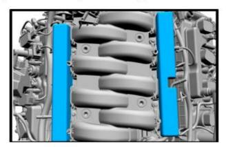
Loosen the (4x) bolts holding the fuel rails down, these go through to the cylinder head (10mm socket). Fuel rail
