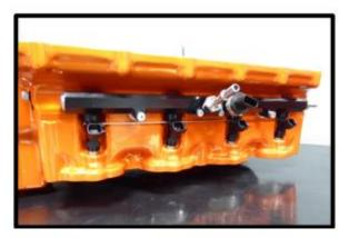
Install supplied 3/8" fuel cross over line around back of the supercharger by pressing until they click and lock in place. \*NOTE: The 90deg end goes to LH side.
