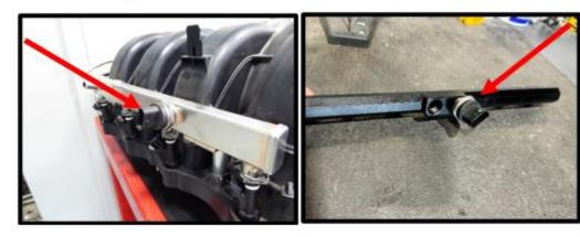
Install supplied (2) #2-906 Viton oring to (2x) 45mm long 9.49mm fuel fittings. Apply light amount of grease to oring for ease of installation and install fitting. Install fittings, one per rail.
