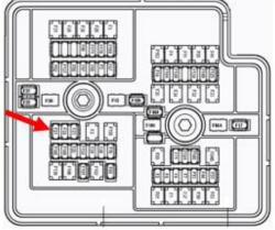
131. Use small set of cutters or file, make a small notch in fuse box cover lid and fuse box to allow wire to fit.
