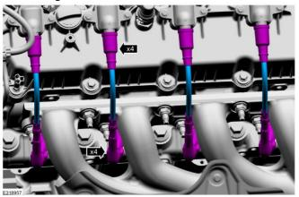
Additional Note: Spark plug torque is 133 lb\*in (15 Nm)
